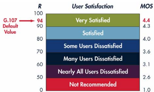
Figure 1. R factor values from the E-model are shown on the left, with MOS values on the right. The likely opinion of human listeners is shown in the middle.
